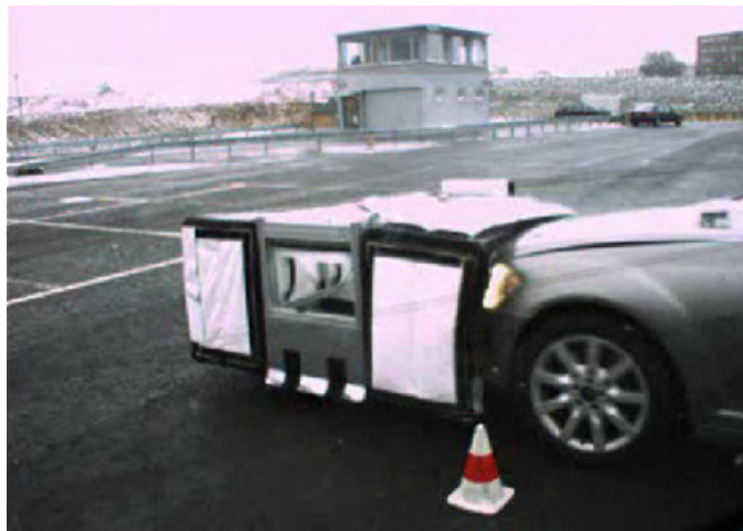
Figure 1: Car impact test at 40 km/h into a 200 kg box behind a vented air cushion (with courtesy to Daimler)
